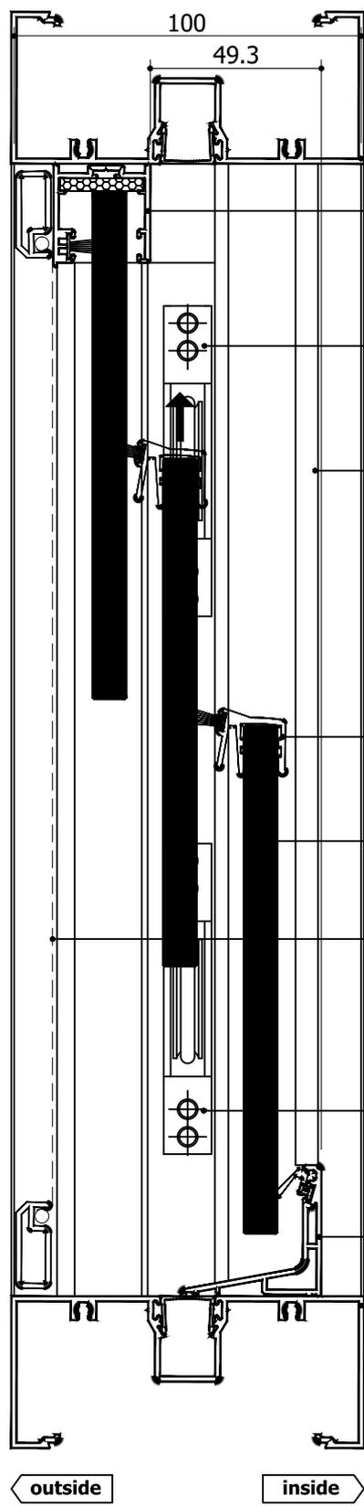
$$\text{glass height} = (\text{opening} + 114\text{mm}) / 3$$
