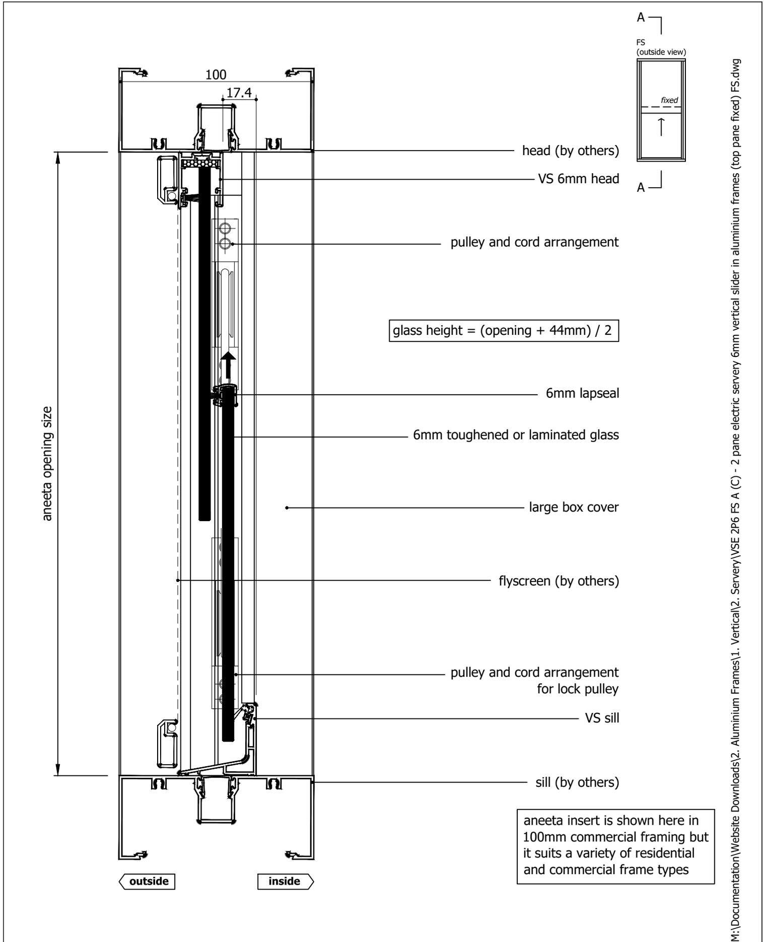
M:\Documentation\Website Downloads\2. Aluminium Frames\1. Vertical\2. Servery\VSE 2P6 FS A (C) - 2 pane electric servery 6mm vertical slider in aluminium frames (top pane fixed) FS.dwg
