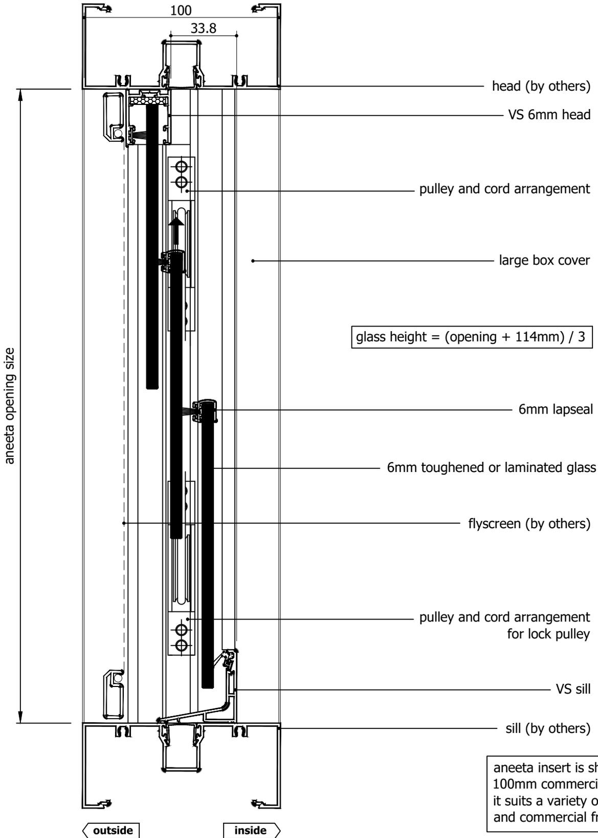
M:\Documentation\Website Downloads\2. Aluminium Frames\1. Vertical\2. Servery\VSE 3P6 FSUF A (C) - 3 pane electric servery 6mm vertical slider in aluminium frames (middle pane sliding up) FSUF.dwg
