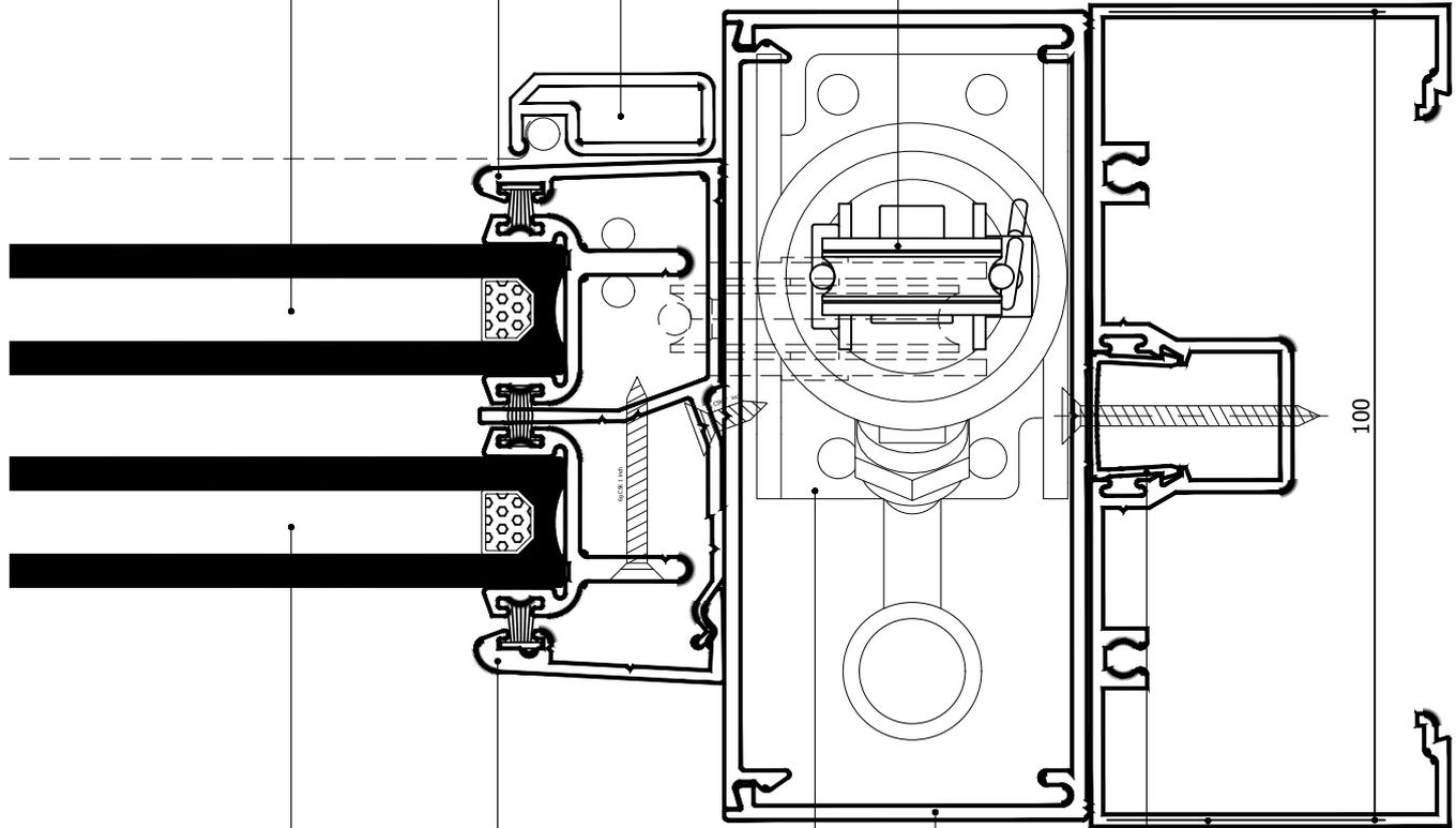
M:\Documentation\Website Downloads\2. Aluminium Frames\1. Vertical\2. Servery\VSE 2P16 SF A (C) - 2 pane electric servery 16mm double glazed INTERLOCKING vertical slider in aluminium frames (bottom pane fixed) SF.dwg
