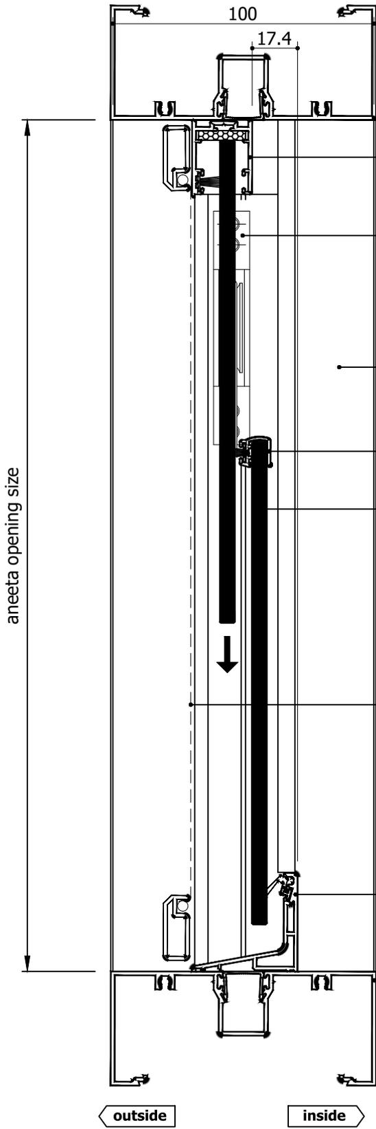
$$\text{glass height} = (\text{opening} + 44\text{mm}) / 2$$
