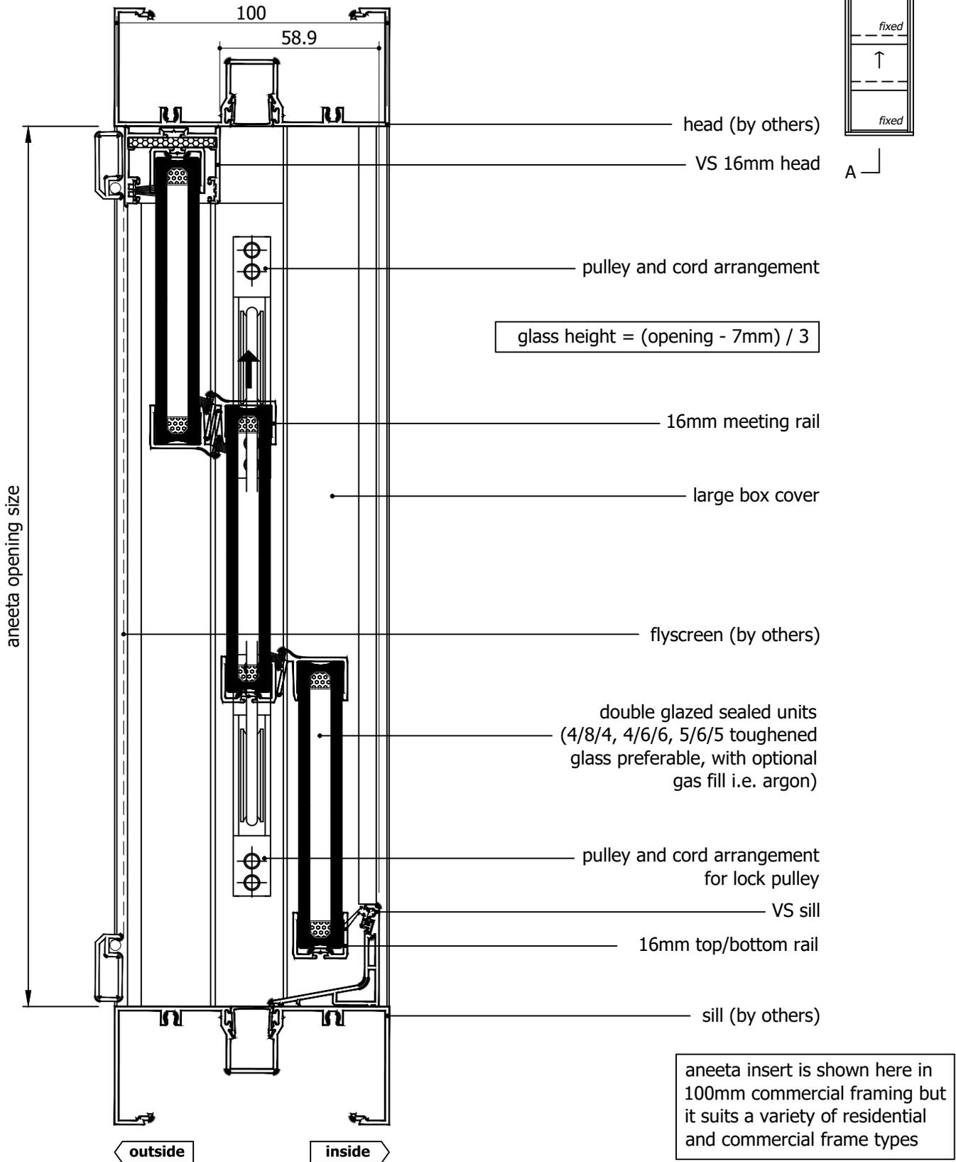
M:\Documentation\Website Downloads\2. Aluminium Frames\1. Vertical\2. Servery\VSE 3P16 FSuF A (C) - 3 pane electric servery 16mm double glazed INTERLOCKING vertical slider in aluminium frames (middle pane sliding up) FSuF.dwg
