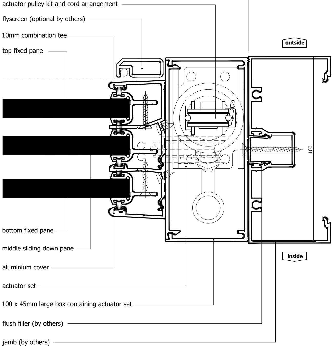
actuator pulley kit and cord arrangement
